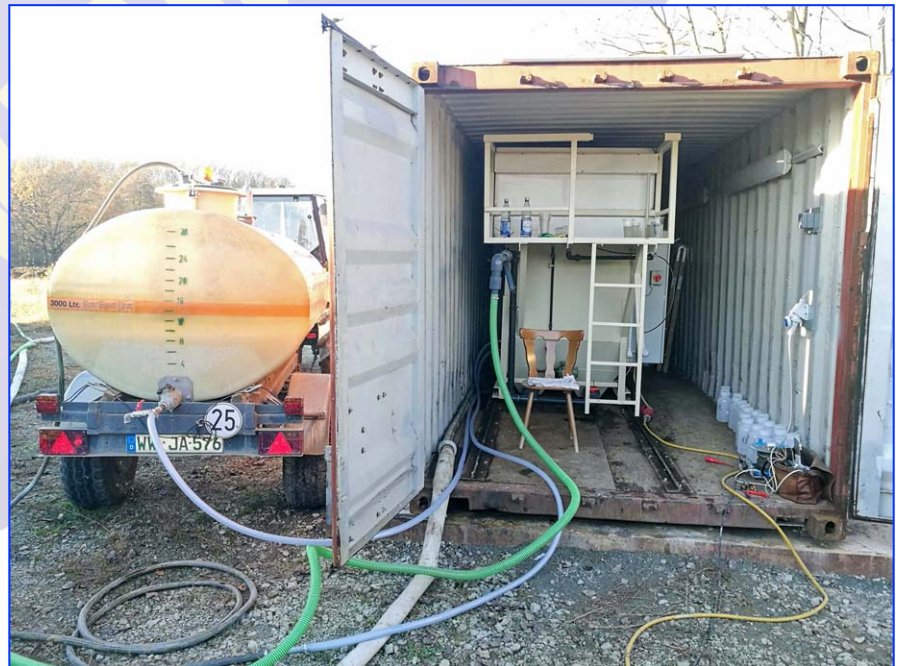
Trial EC Plant, 1 m 3 /hr c/w settlement clarifier all within a shipping container for on-site trials
