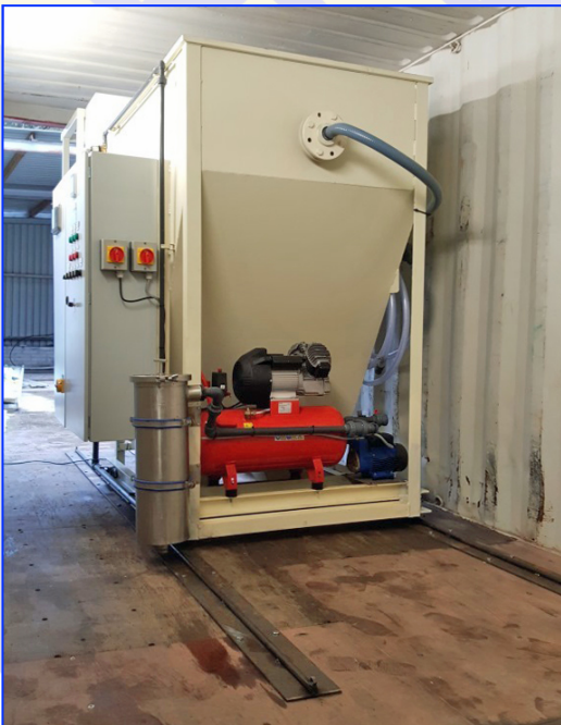
Trial EC Plant, 1 m 3 /hr c/w settlement clarifier all within a shipping container for on-site trials
