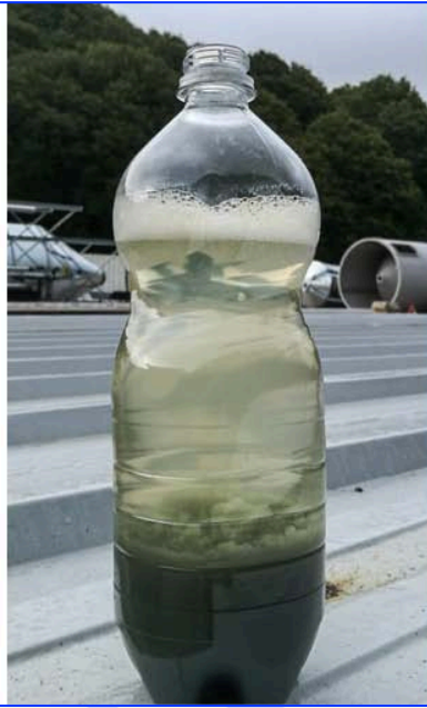
After EC treatment & settlement. Sludge settles in 15 mins leaving treated clear water above.
