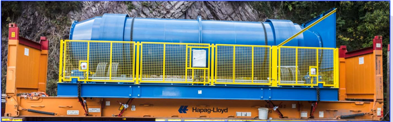
PulpStar 5 on flatpack ready for shipping. Capacity 5 tonnes per hour MSW
